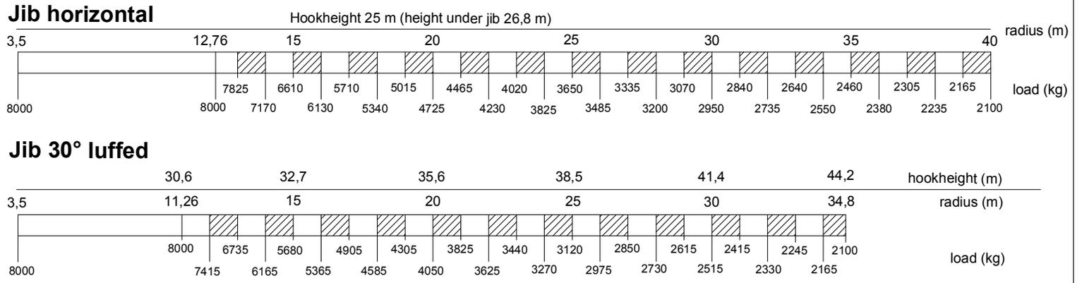
**LIFTING CHART Outrigger spread 6,90 m x 5,15 m**
